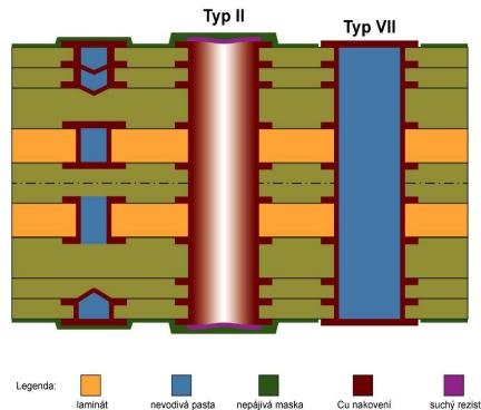
If not stated otherwise, all through holes (VIA) are always filled up to drill diameter of 0.45 mm. It is ideal to specify the diameter of the hole that the customer requires to be filled, or to indicate the maximum diameter of the filled holes. If you want to fill only the selected holes (area), you must specify them in a separate layer, or in the attached drawing.
